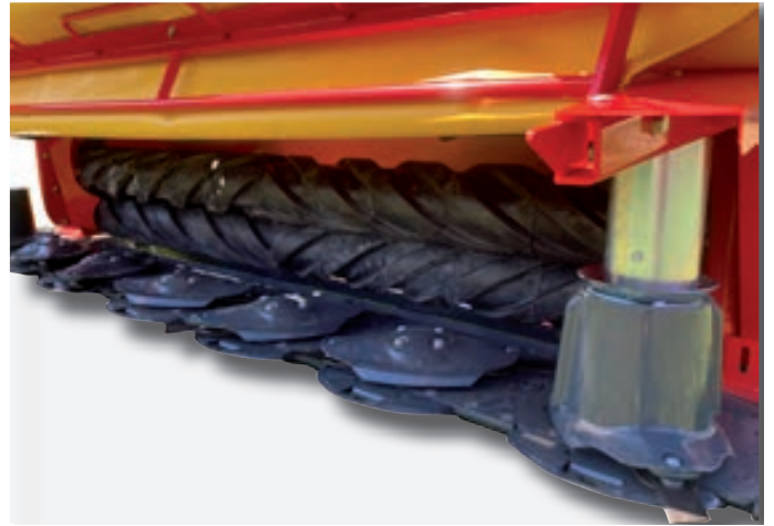
Roller conditioner of model SC-301R.
