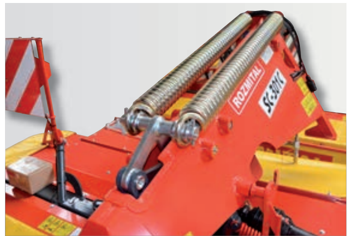
Cutterbar flotation by using springs.
