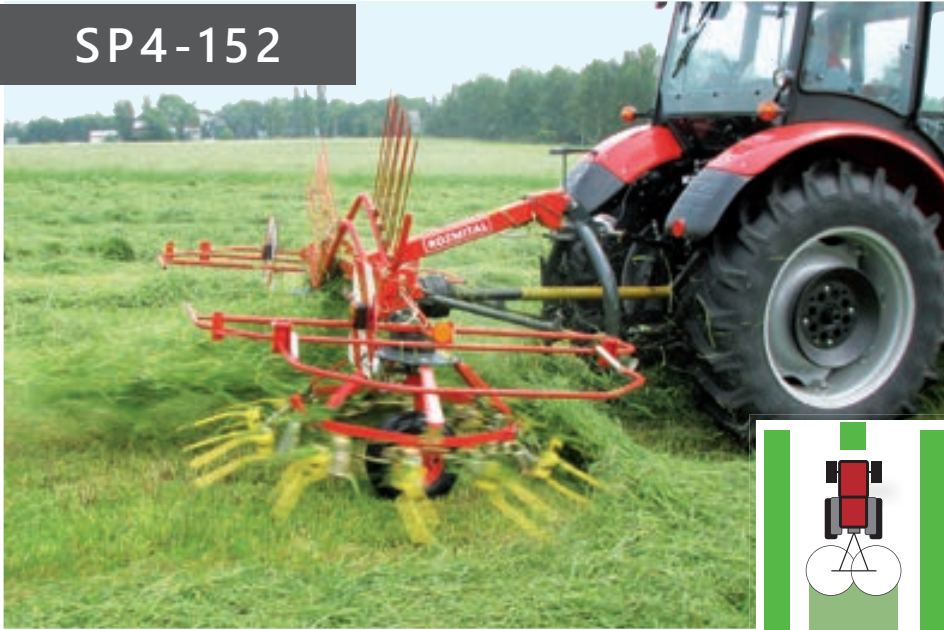
Tedding - rod swath guards are in transport position.
