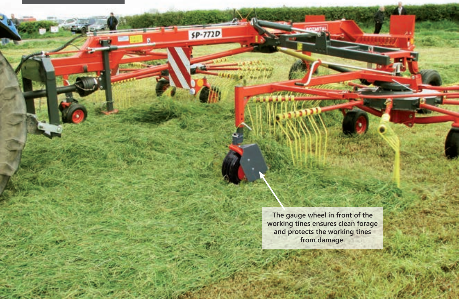
SP - 772D mid-row two rotor rake with incrementally adjustable working width
